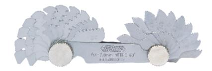
■ Check the pitch of screw thread
